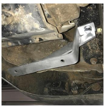
4. Attach the skid plate to the two vertical brackets using the M8 bolts + flat washers on both sides of the Skid plate + nyloc nuts on the top side.
