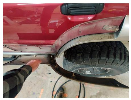
Again, just clips on this panel. Pry and pull, pry and pull.
