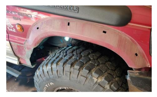
On the back passenger doors, there is a screw at this location that needs removal before prying.
