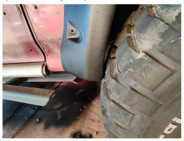
Matching bedliner vinyl wrap by sanding and spraying flares with bedliner coating
