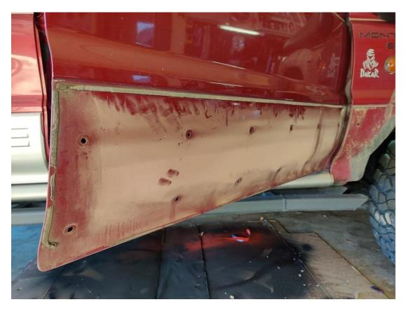
There are several screws and tabs to remove on the under side of this panel. After that, just pry and pull.
