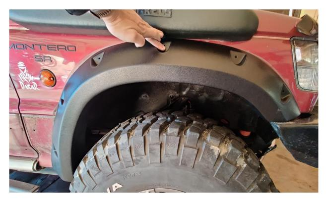
\*\*Treat exposed metal after drilling to help with rusting.
