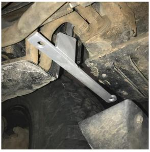
3. Install the rear bracket (thicker of the two brackets) into the second from the rear threaded mounting hole in the chassis using the M12 bolt + locker washer + flat washer. This will work even if you have an aftermarket tow hitch:
