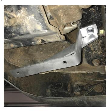
4. Attach the guard to the two vertical brackets using the M8 bolts + flat washers on both sides of the guard + nyloc nuts on the top side.
