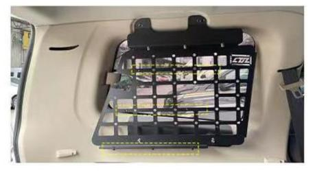
6. Horizontal Shelf Installation (if applicable) – There are 4 available positions (Upper, Middle, Lower, and Front/Vertical). Install the angle iron bracket using the provided wing bolt hardware. \*Not needed for the Lower position as the bracket can be attached directly to the side panels.
