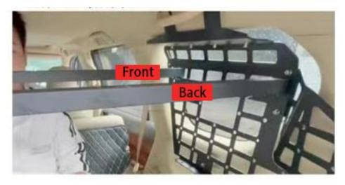
9. Place the shelf halves under the crossbars and onto the side brackets.
