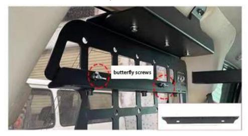
7. Crossbar Orientation – The front bar has 4 hole that need to face forward and 6 downward. The rear bar's 6 holes will all face downward. See step 11 for an illustration.
