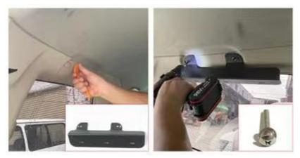
3. Hang the side panel on the upper bracket, line up the bottom bracket with the 2 corresponding bolt holes on the side panel and mark its location on the vehicle.
