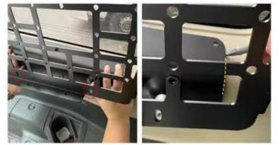
4. Remove the side panel, use an included adhesion promoter to wipe the installation area, then affix the bottom bracket along the mark drawn in step 3, and then press firmly.
