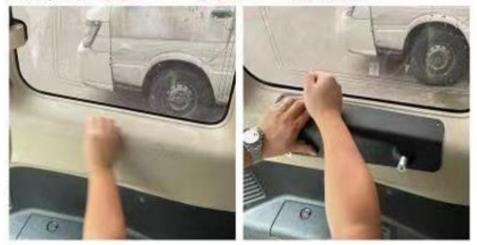
5. Attach the side panel to the top and bottom brackets loosely and then once all bolts are installed they can be tightened. The side panel installation is now complete.
